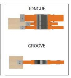
Each function of the 6 piece cope & pattern set requires a different cutter configuration. For desired results, use the following guide to set up each operation.
